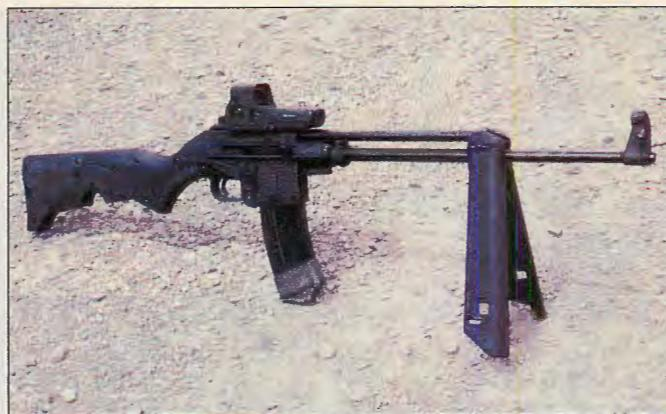
The Aimpoint Comp ML2 Sight was mounted on the SU-16 using the new mount from World Wide Ordnance. WWO's extended-eye-relief mount is also shown. (below) As a compact weapon, the SU-16D compares favorably with an M4 in the collapsed mode.
